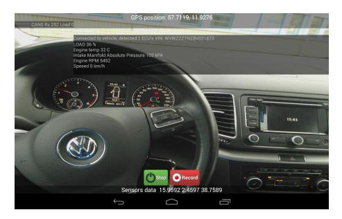
The option automatically reads our important data such as VIN number and status of the electronic units, when connected to a vehicle. DTC's can be followed on a single service level or per ECU.
