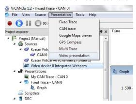
Assign the source to its presenter. Just as with the CAN (or any source in ViCANdo) sources before
