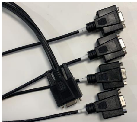
Figure 4 1F4F split cable
